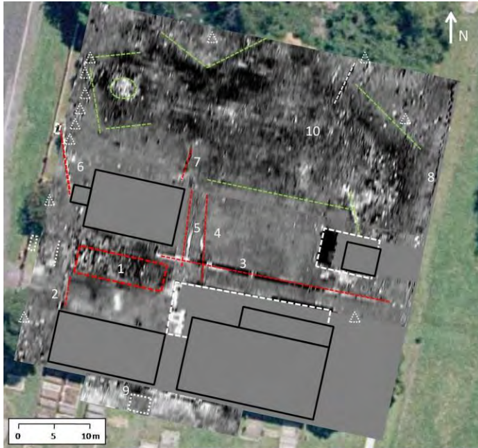
Figure 3.83 Methodist Church Group. Ground penetrating radar image showing the location of a former structure (dashed rectangle 1) (possibly the site of the second 1919 chapel) and services (dashed lines). The report notes that area No 10 to the north of the church contains a well and could possibly contain the remains of brick foundations and other structures (possibly the site of John Lees' second house). (Source: Archaeological Computing Laboratory, University of Sydney, 2008)
